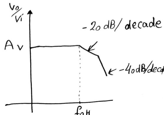
\* The circuit voltage gain and cutoff frequency are the same for the second order circuit as for the first order filter circuit except that the filter response drops at a fast rate a second order filter circuit.
