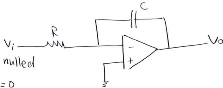
$$V_o(t) - V_o(0) = -\frac{1}{RC} \int_0^t V_i dt$$
