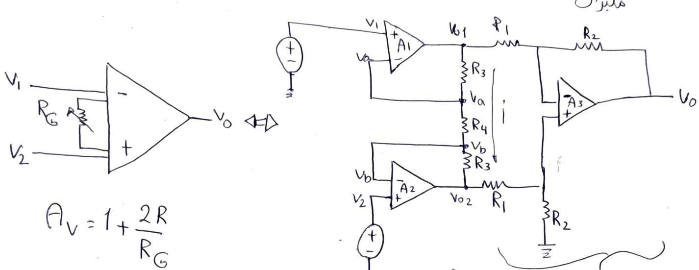
$$A_V = \frac{R_2}{R_1} \left(1 + \frac{2R_3}{R_4}\right) \text{ مكثف}$$
