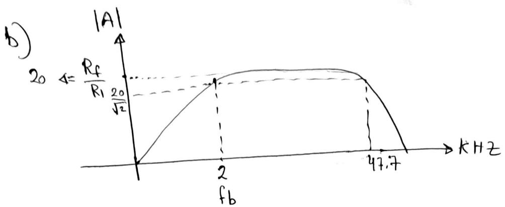
$$\frac{R_f}{R_1} = \frac{15.9 k\Omega}{796 \Omega} \approx 20$$
