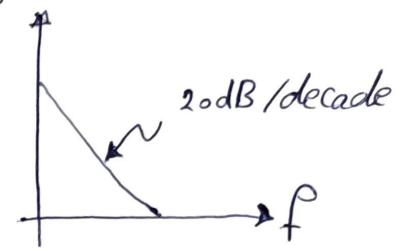
$$V_i = A \sin \omega t \Rightarrow V_o = \frac{1}{R_1 C} \int A \sin \omega t \cdot dt$$
