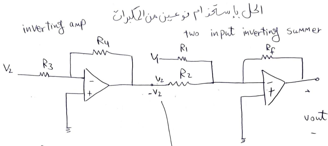
$$R_4 = R_3 = 10 \text{ k}\Omega$$
