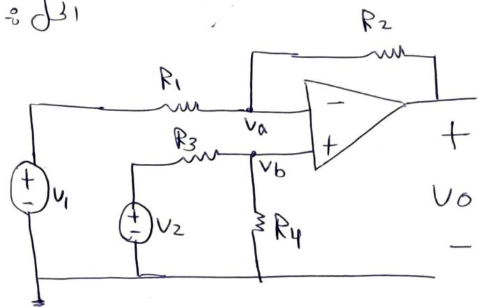
$$R_1 = 10\text{k}\Omega \quad \text{نفرض} \\ \therefore R_2 = 50\text{k}\Omega$$
