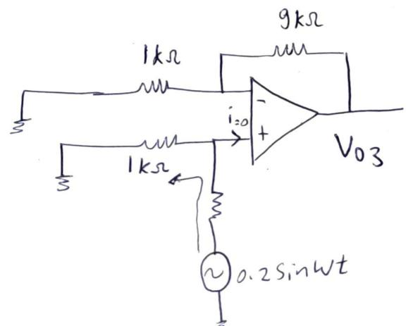
$$\therefore V_o = V_{o1} + V_{o2} + V_{o3}$$
