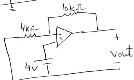
$$\text{OR by using KCL} \quad \therefore \frac{6 - V_1}{4k\Omega} = \frac{V_1 - V_o}{10k\Omega}$$
