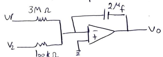
$$V_o(t) = -\frac{1}{R_1 C} \int_0^t V_1 dt - \frac{1}{R_2 C} \int_0^t V_2 dt$$
