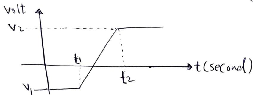
$$\text{rate change of op amp function} = \frac{V_2 - V_1}{t_2 - t_1}$$
