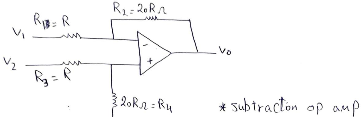
$$\therefore \frac{R_1}{R_2} = \frac{R_3}{R_4}$$
