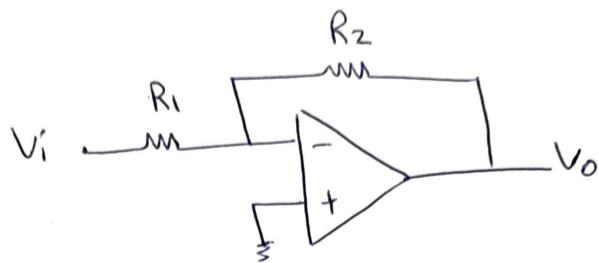
use resistors no larger than  $1 M\Omega$ . Design the circuit having the largest possible input resistor.
